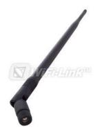
This compact 7dBi 2.4GHz OMNI directional "rubber-duck" WiFi antenna provides broad coverage. It is ideally suited for IEEE 802.11b and 802.11g wireless LANs, This flexible antenna features a tilt-and-swivel reverse-polarity SMA connector, allowing them to be used vertically, at a right angle, or any angle in-between. It is a replacement for RF Reverse Polarity SMA connectors Antennas on the access points or radios and routers, such as D-Link®, Linksys® WET11 and others.
